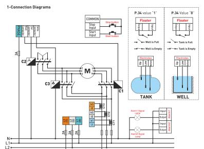
**Note:** To control the level of liquid in the well by electrodes, make connections according to figure 1. Connect floter to the tank. Adjust **Pr.34** to 0.
